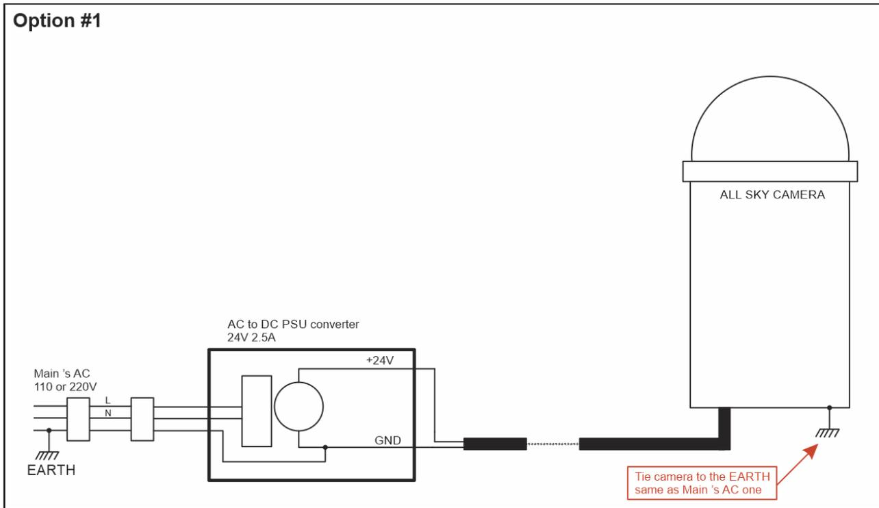
Fig. 105 System grounding scheme (Option 1)
