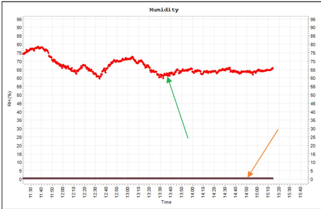
Fig. 94 Relative humidity plot, the orange arrow shows the inner humidity level of the camera. Here close to zero on a brand-new camera with fresh desiccant.
