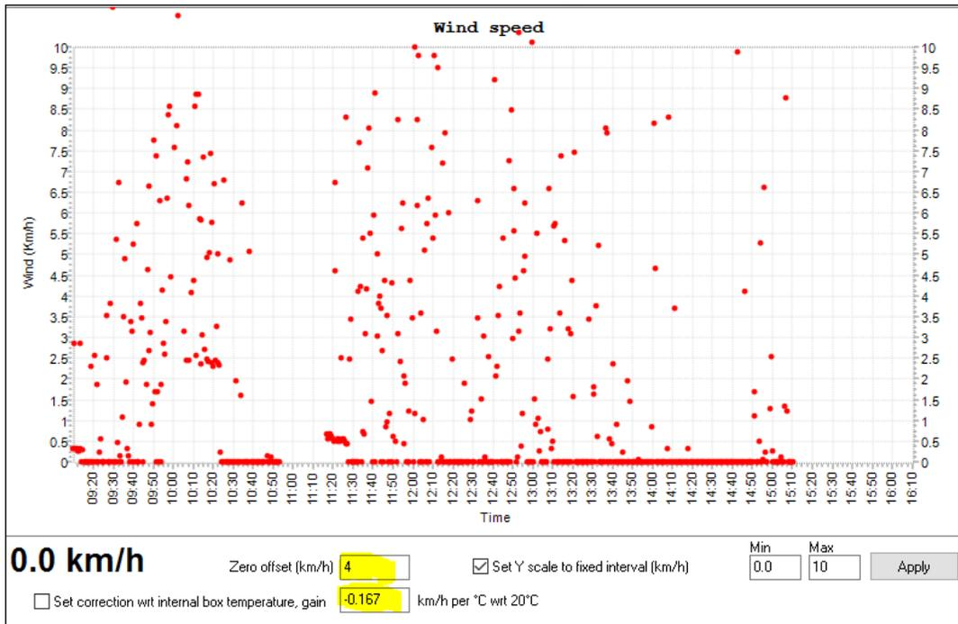
Fig. 102 Wind speed plot
