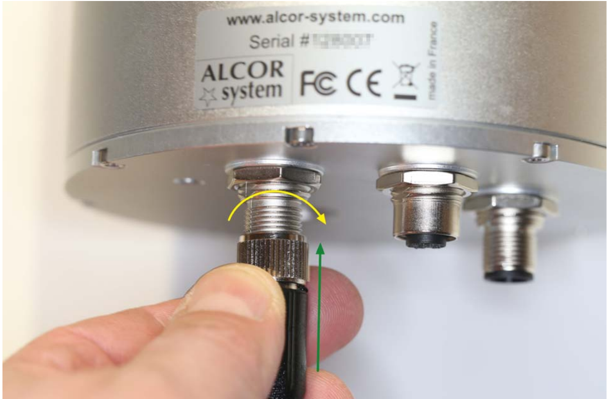
Fig. 11 Spot the coding notch and push the cable connector, then rotate several turns to screw it.
