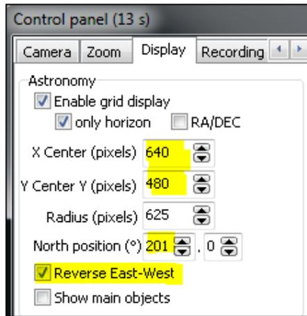
Fig. 76 displacement in X and Y to adjust the position of the zenith symbol
