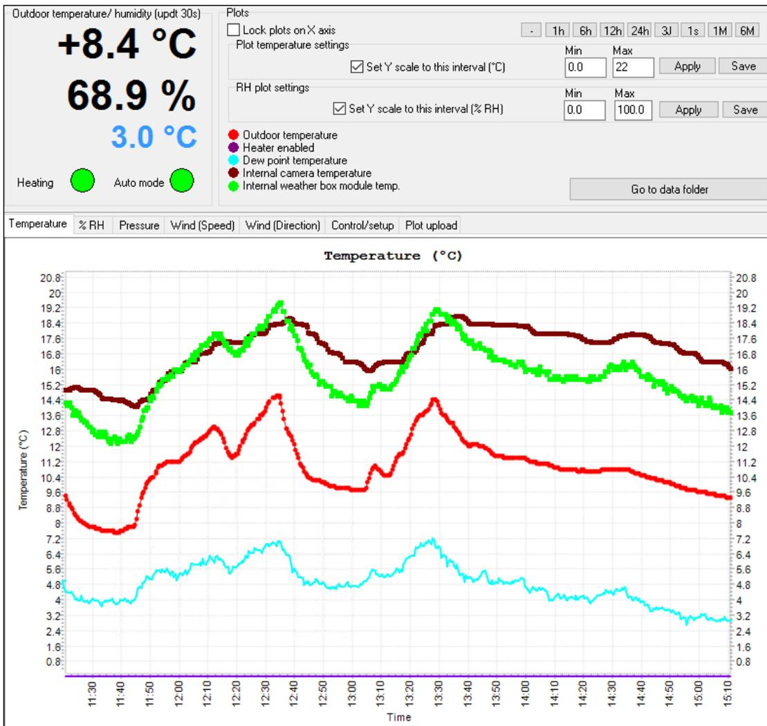
Fig. 101 Temperature from the different sensor of the camera. Red is external temperature, brown is internal camera temperature, green is weather box internal temperature, and cyan is the dew point temperature.
