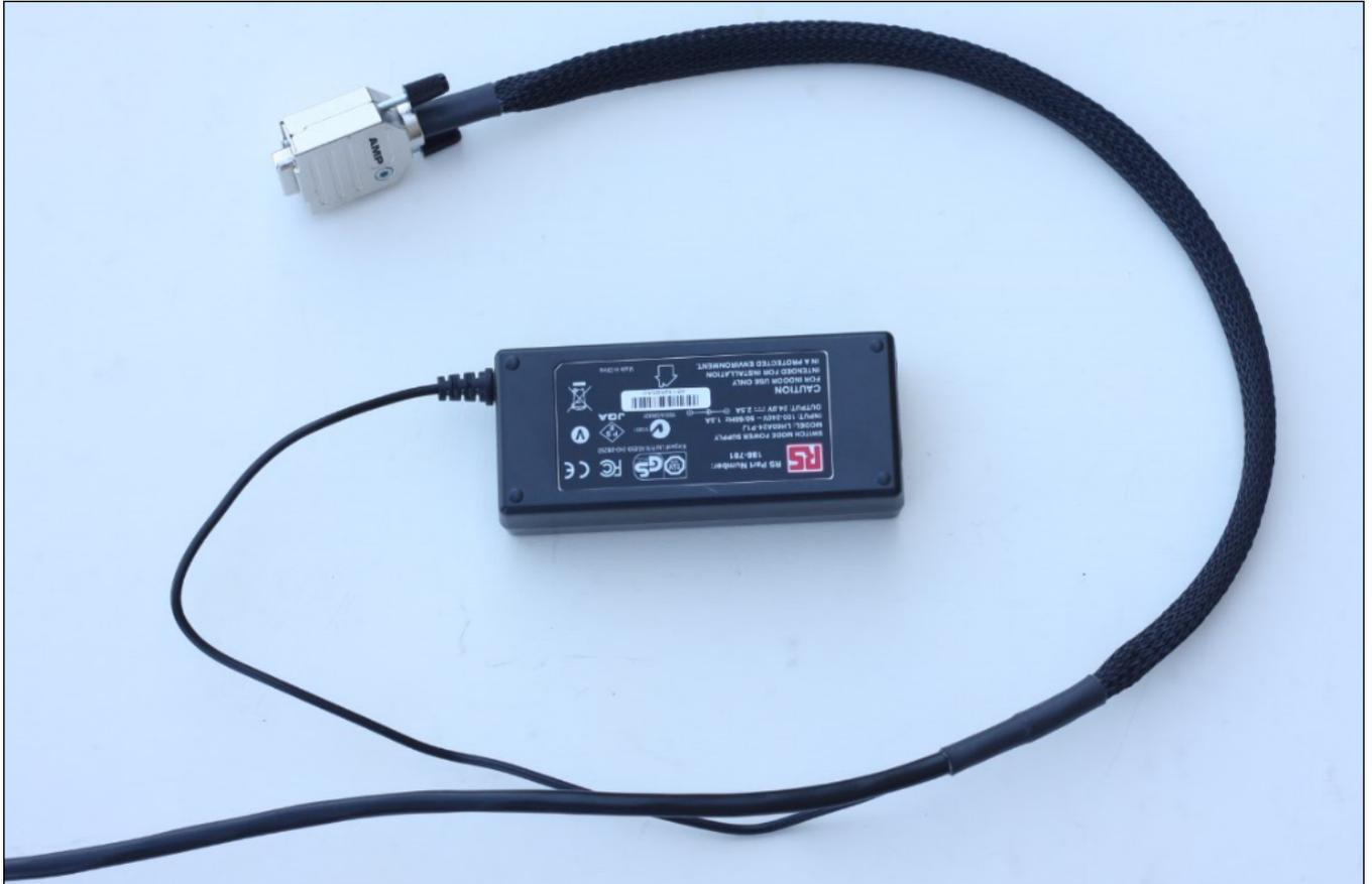
Fig. 16 RS232 connector and 24V 2.5A power
