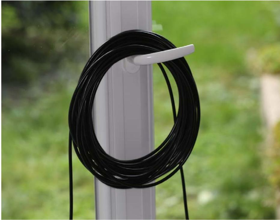
Fig. 13 **Avoid to coil the USB and Power cable this way,**
