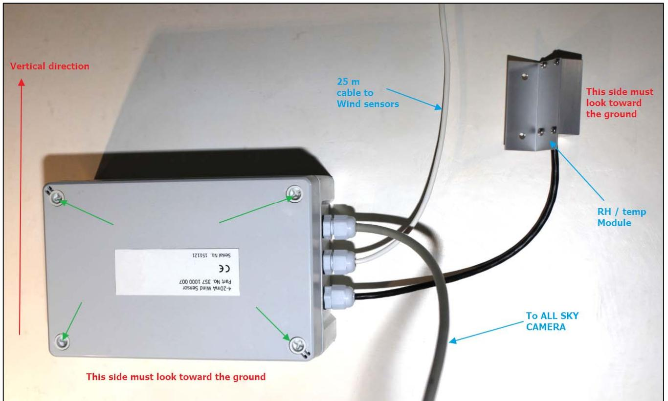
Fig. 98 Sensors control box
