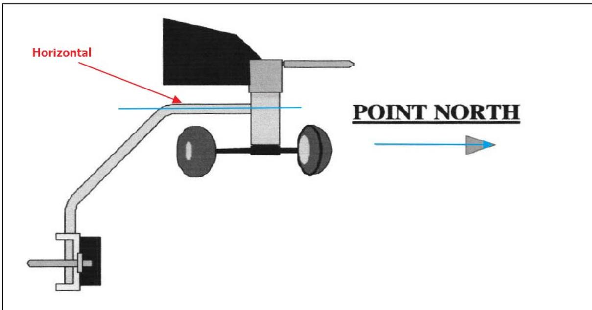
Fig. 99 Wind-sensor orientation
