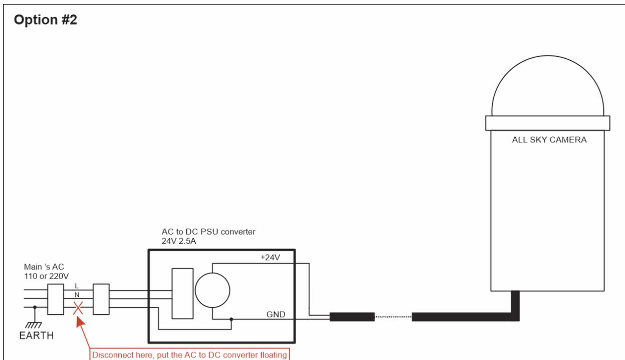
Fig. 106 System grounding scheme (Option 2)
