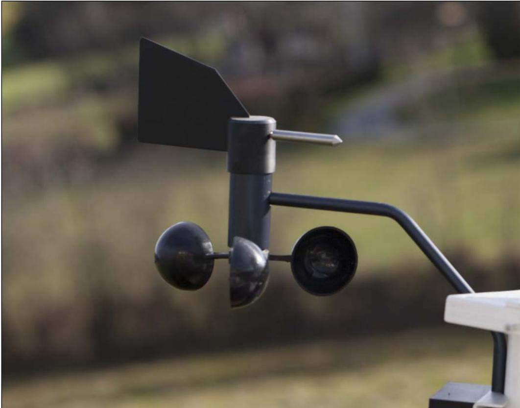
*Fig. 97 Wind speed and Wind direction sensor*
