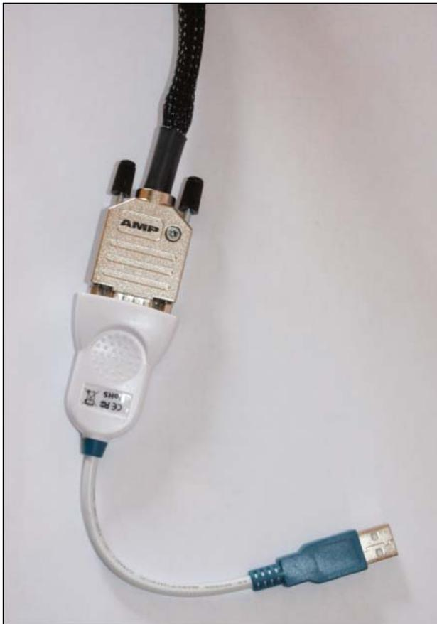
Fig. 18 RS232 to USB converter
