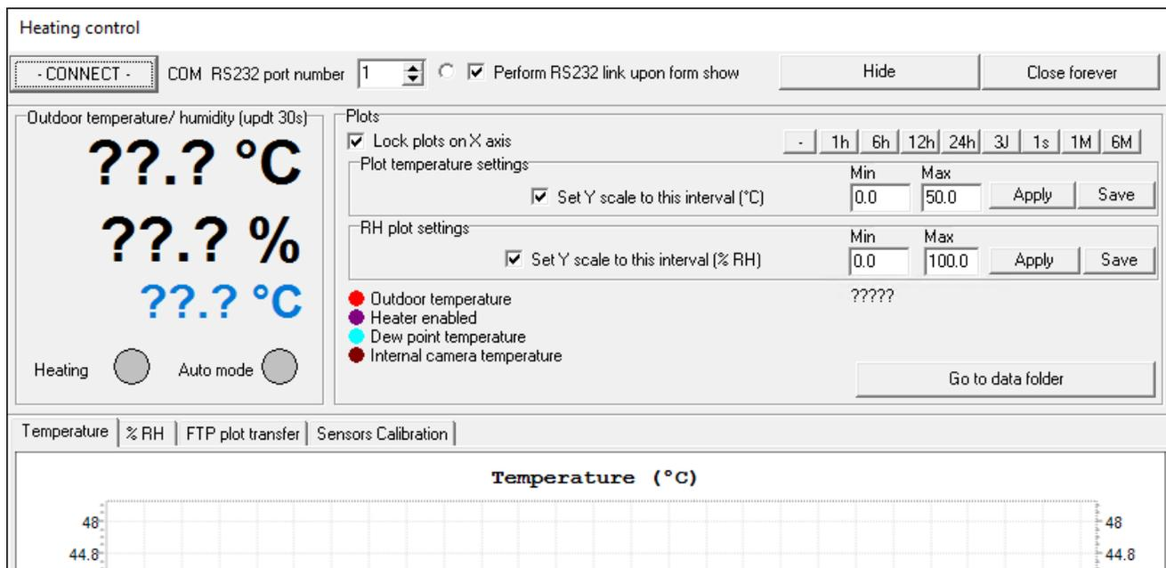
Fig. 36 Heating window software.
