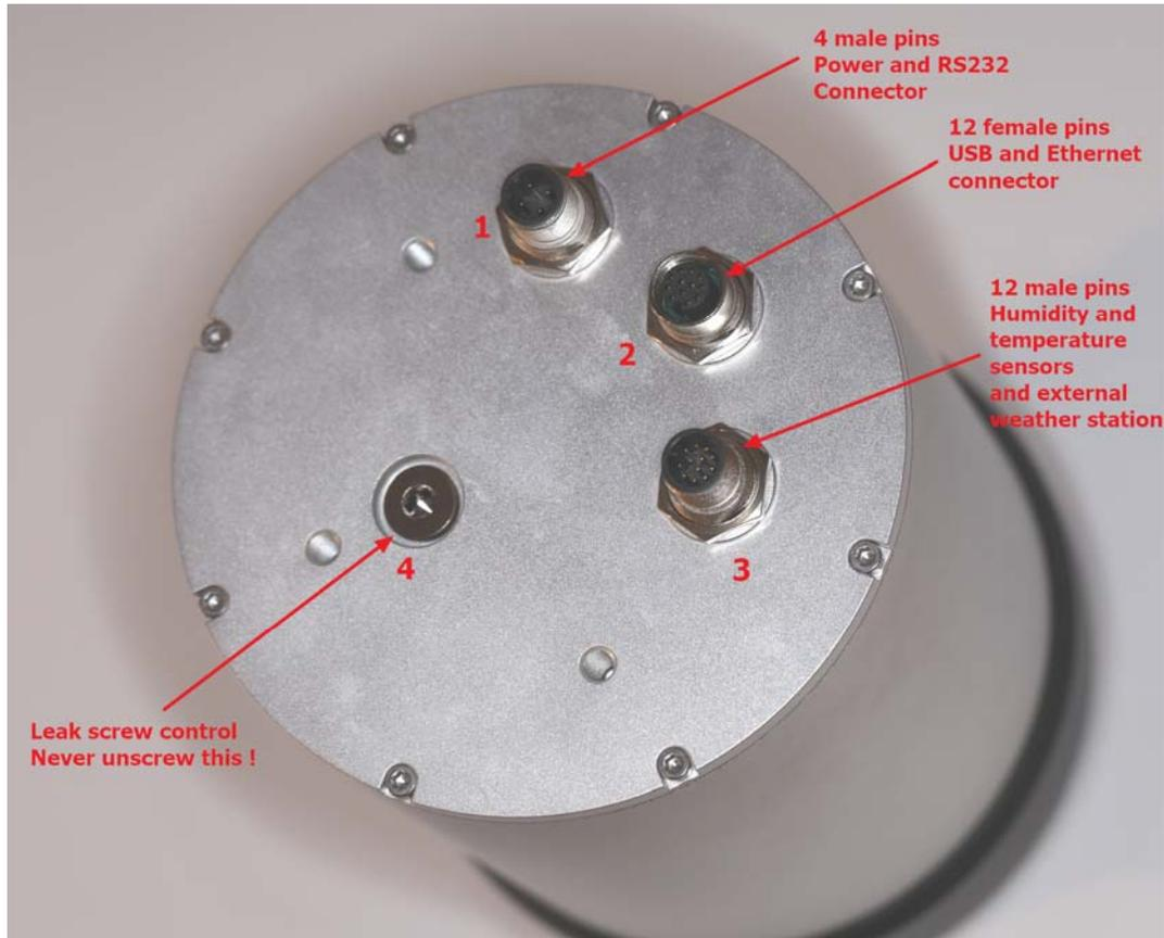
Fig. 9 New metal connectors located at camera backside
