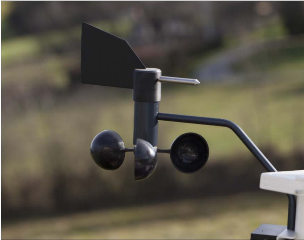
Fig. 99 Wind speed and Wind direction sensor
