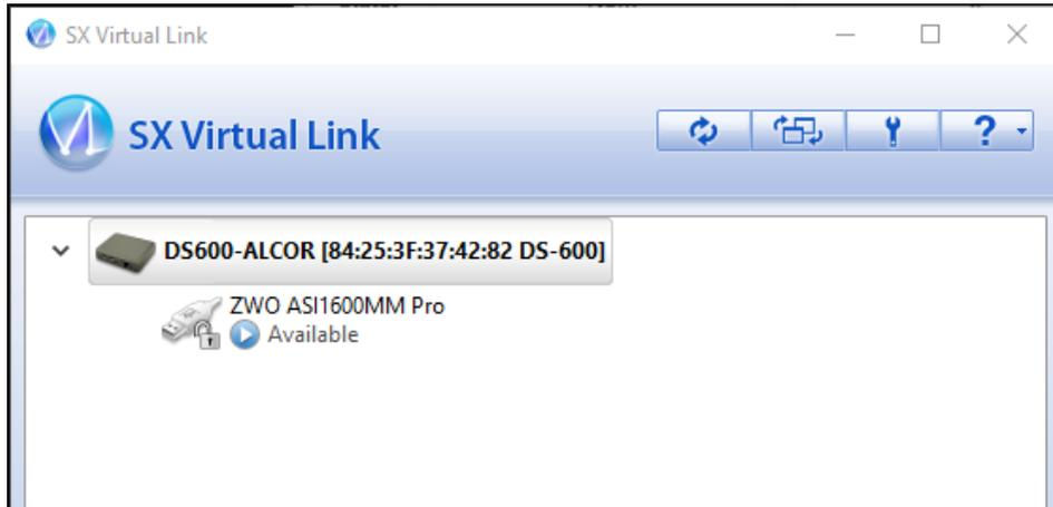
To get the camera connected, right click on the camera and click **“Connect”**
