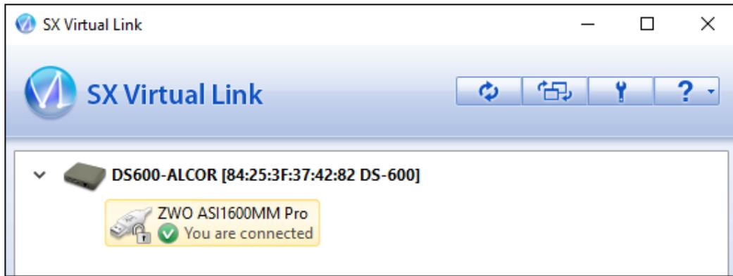
This is possible to auto-connect the camera and the filter wheel, right click on the device, then the pop-up menu shows a property menu. Then go the the “connect” tab.
