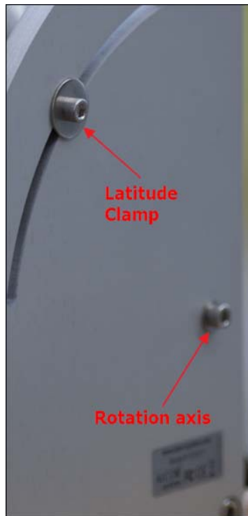
Fig. 19 Latitude clamp, use M6 Allen Key to release it (Cyclope)
