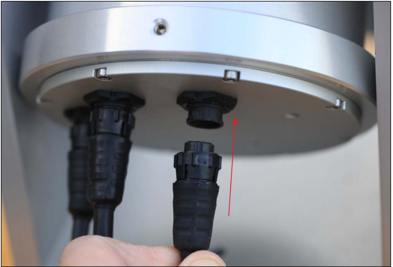
Fig. 8 Push the connector straight
