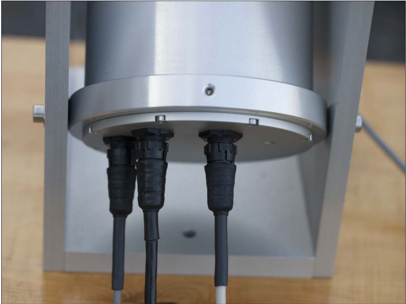
Fig. 6 Three cables, one is going to the temperature and humidity sensor, and other goes to inside a building.
