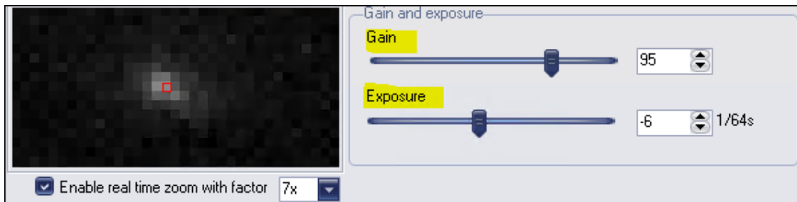
Fig. 67 Exposure time and Gain can be tuned to get the best detection level of Polaris
