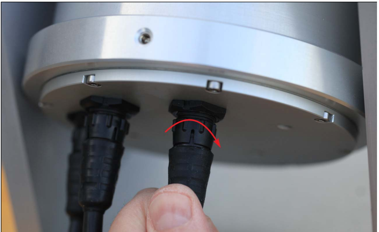
Fig. 9 Then turn the connector's collar in clockwise fashion
