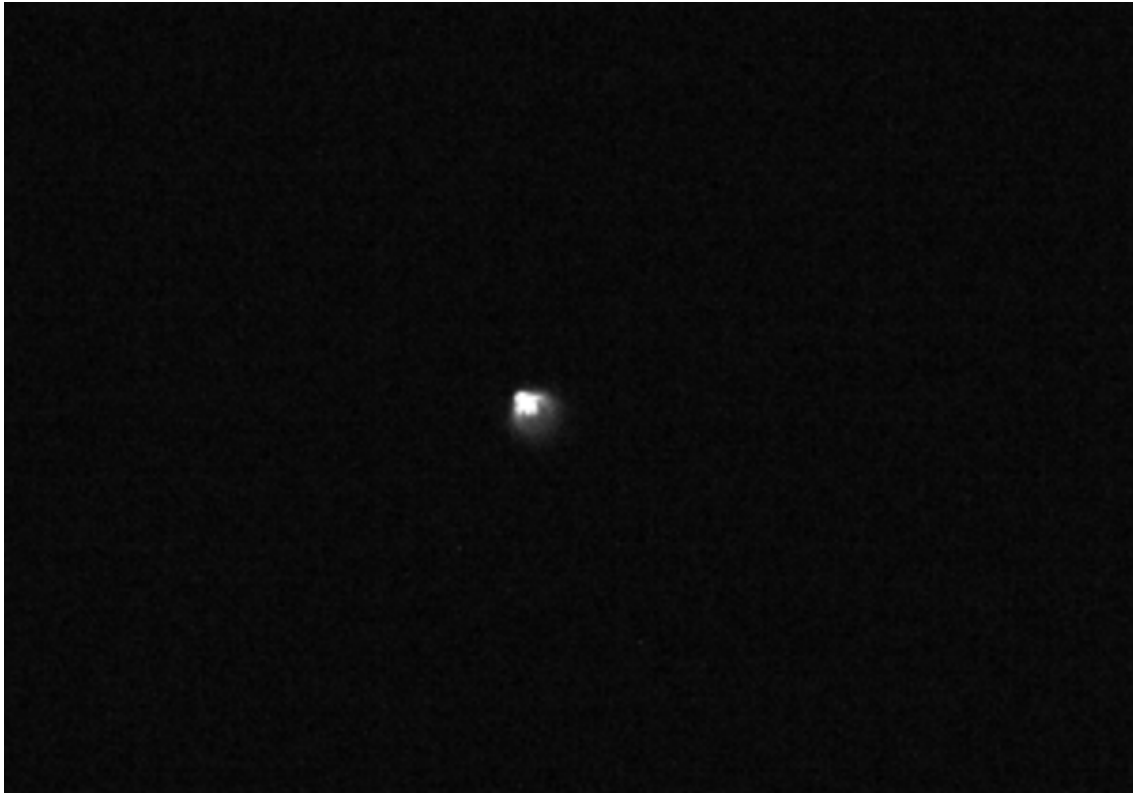
Fig. 69 Long exposure on Polaris (1/7s) showing some filter reflection effect (halo)
