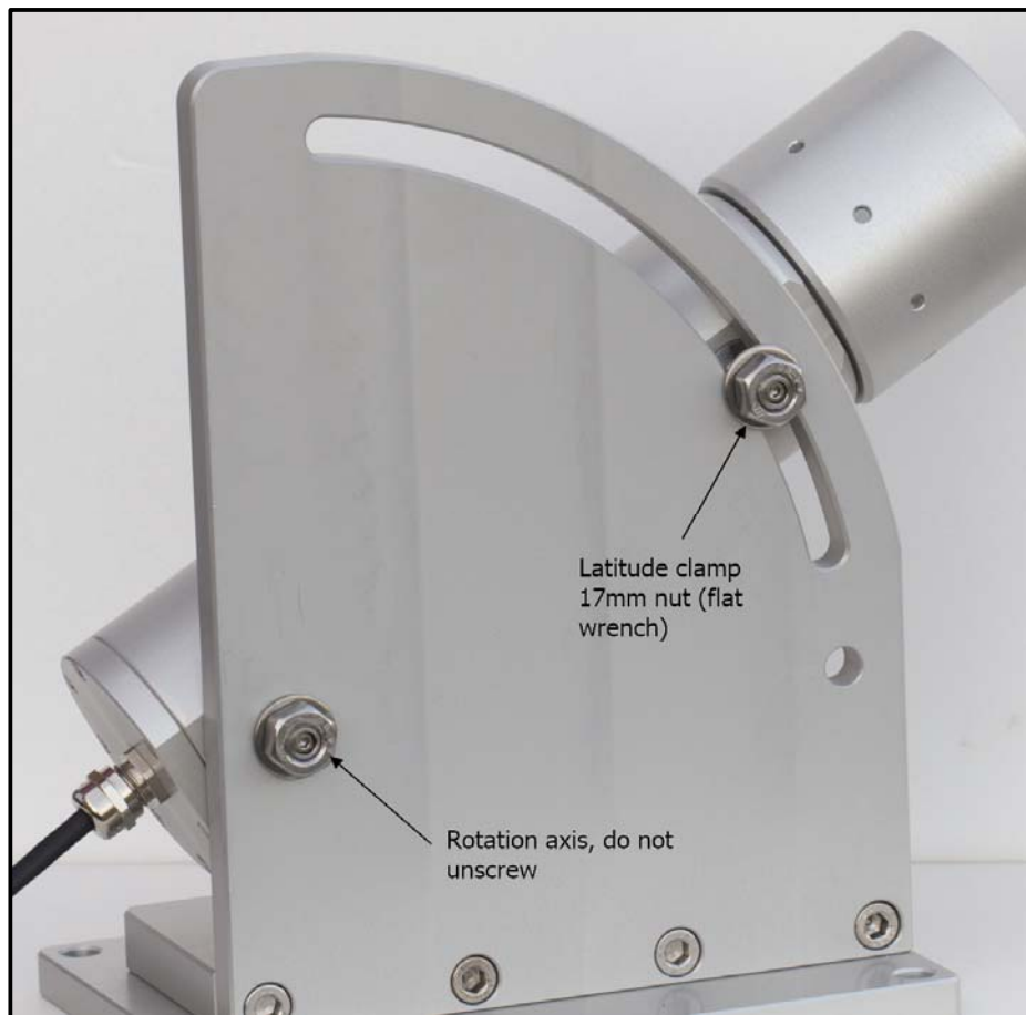
Fig. 20 Latitude clamp, use 17 mm flat wrench to release it ( \mu -Cyclope)
