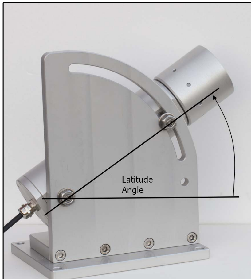
Fig. 18 The angle depicted above has the same value of the local geographical latitude ( \mu -Cyclope)
