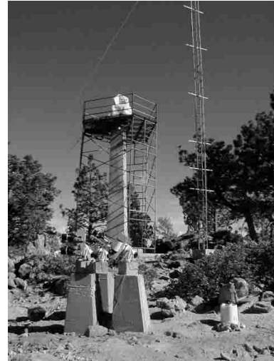
Fig. 1. Layout of the GSM (foreground), of the DIMM tower (left-background) and the mast (right-background).
