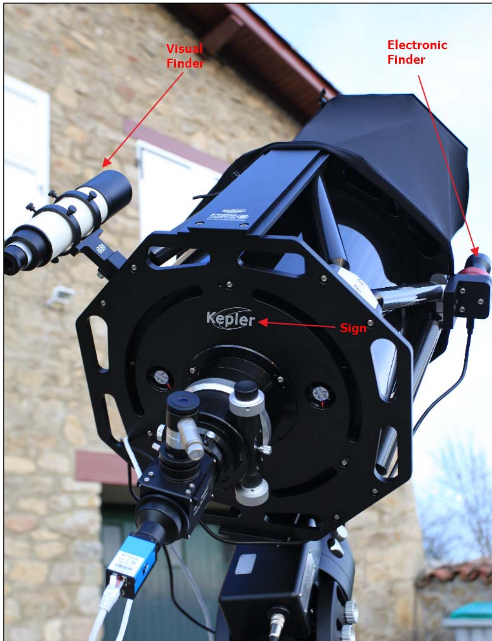
Fig. 3 Orientation of the tube (mandatory)
