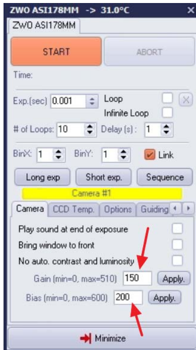
Fig. 53 Check the gain and Bias to these figures.
