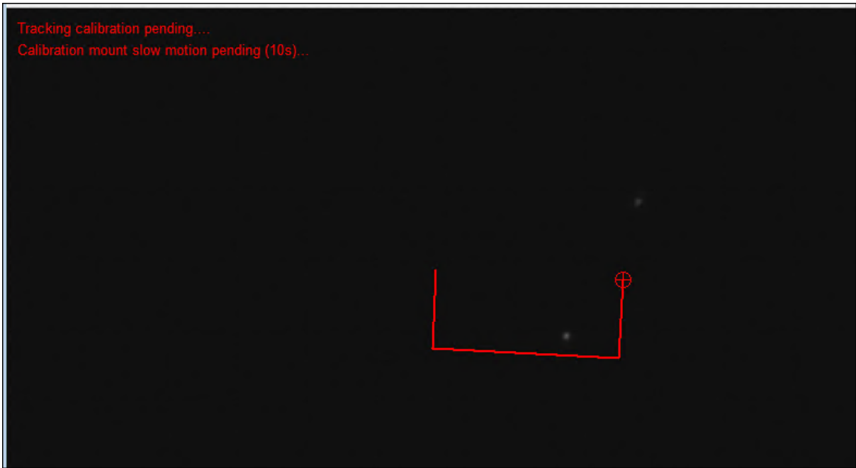
Fig. 95 Calibration pending, RA+, DEC+ and RA- have been achieved
