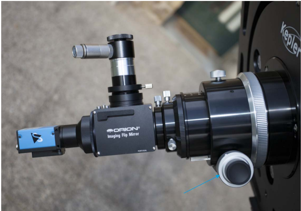
Fig. 65 Focusing knob of the RC telescope
