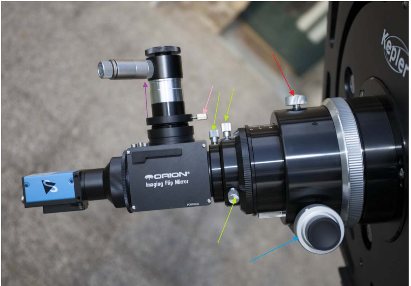
Fig. 68 Screws to be used for setting the best focus for the camera AND the eyepiece at the same time.
