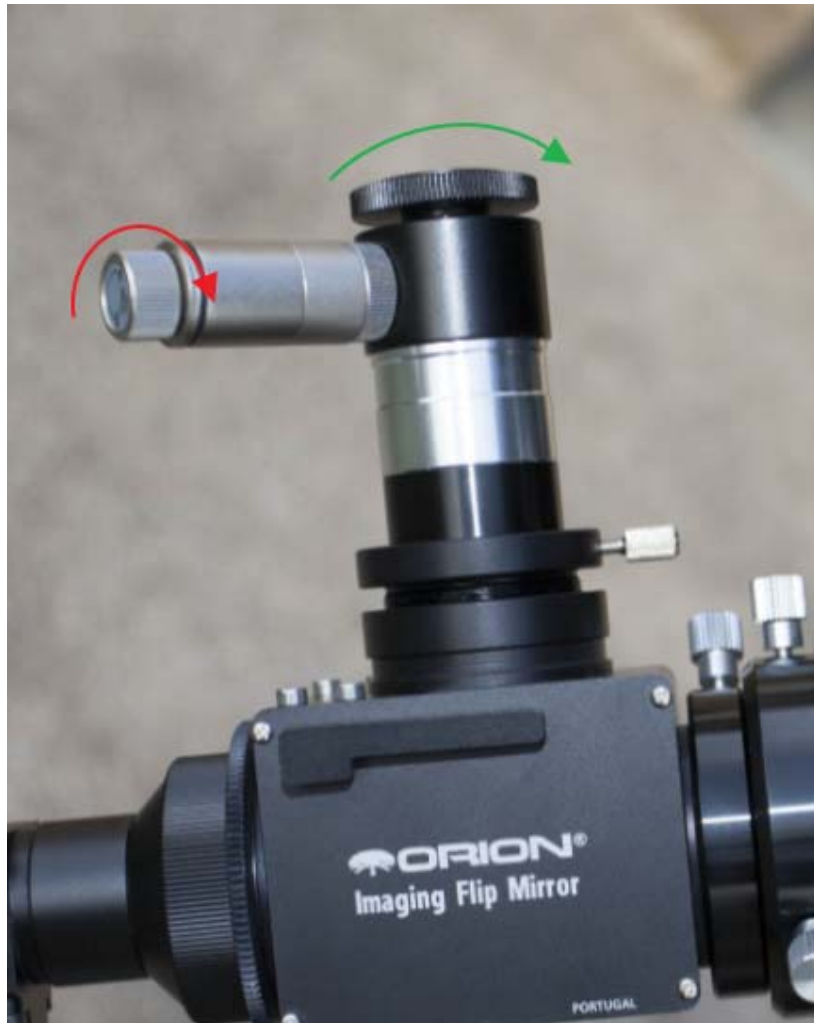
Fig. 15 Reticle eyepiece settings
