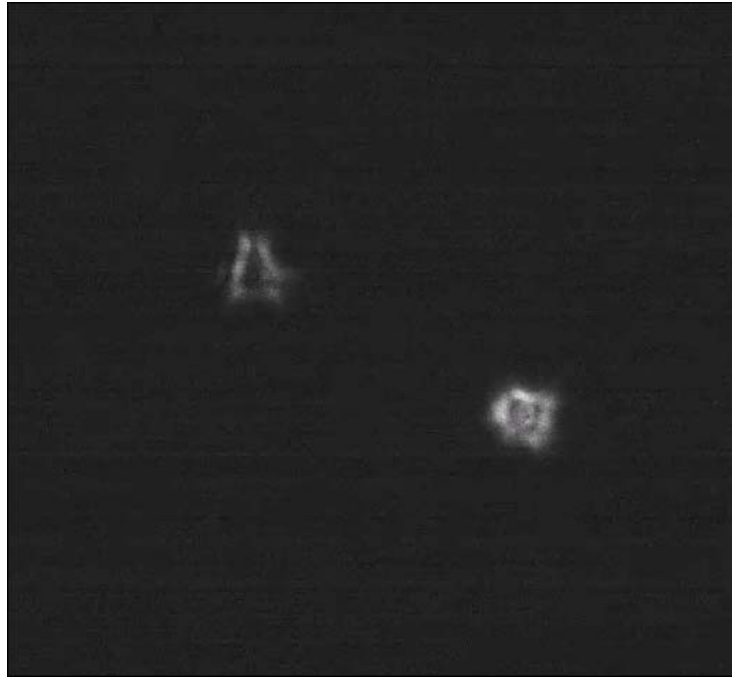
Fig. 64 Unfocused star image, this is not suitable for DIMM measurements
