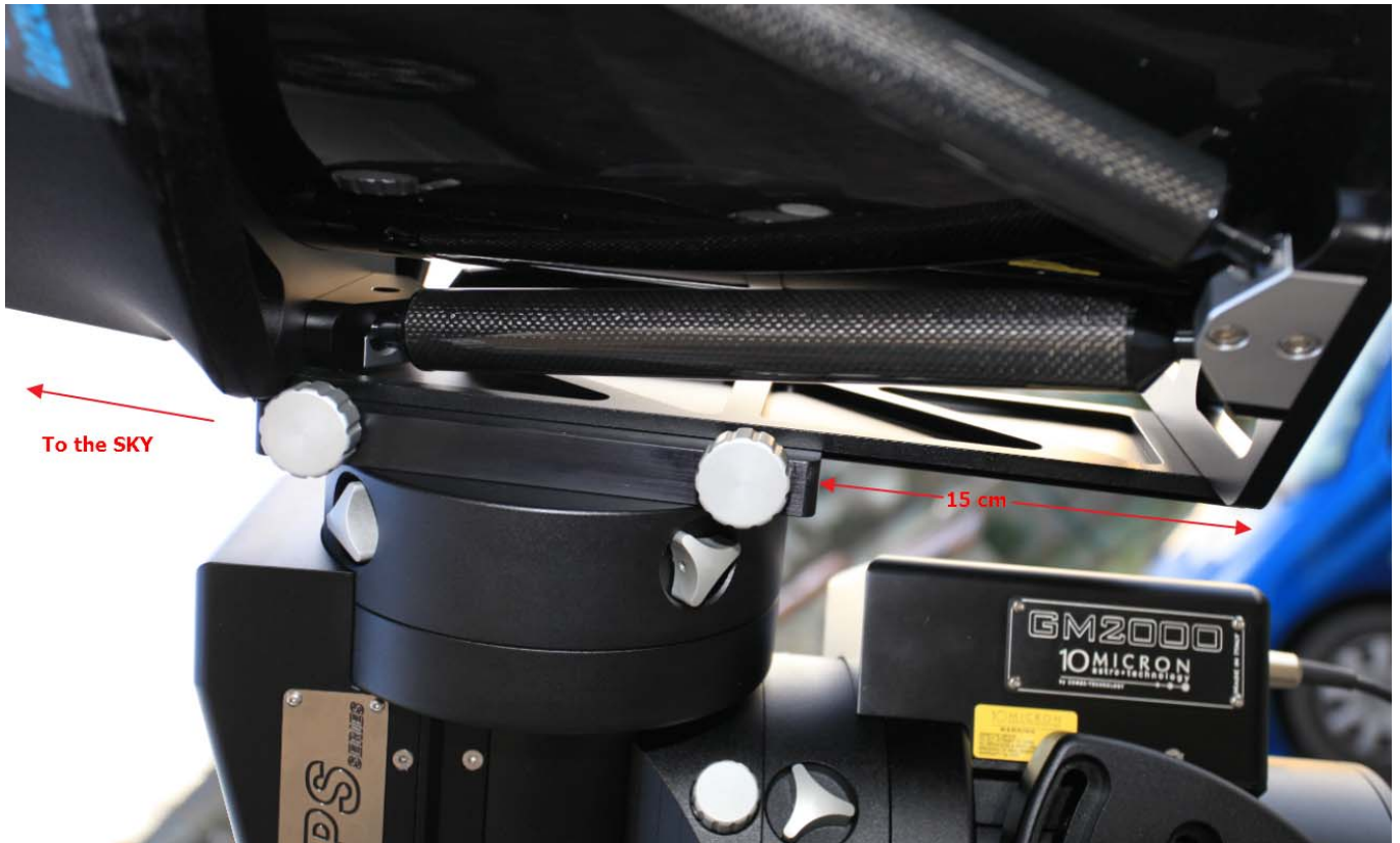
Fig. 4 Tube position for optimum DEC balancing
