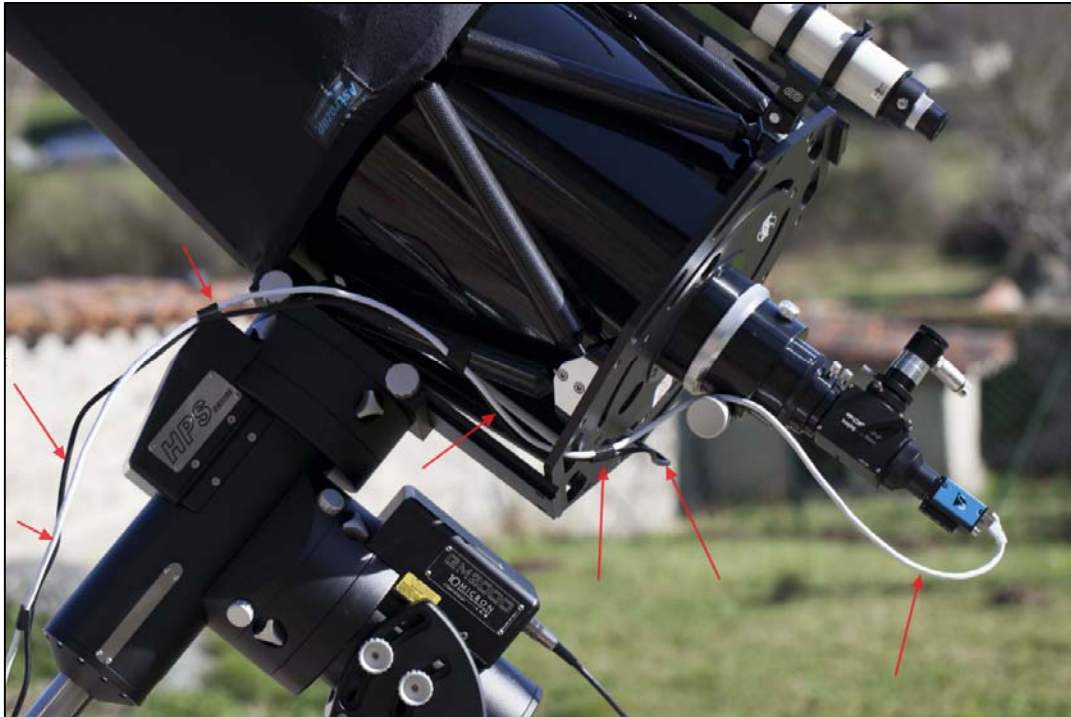
Fig. 19 Path of the cables
