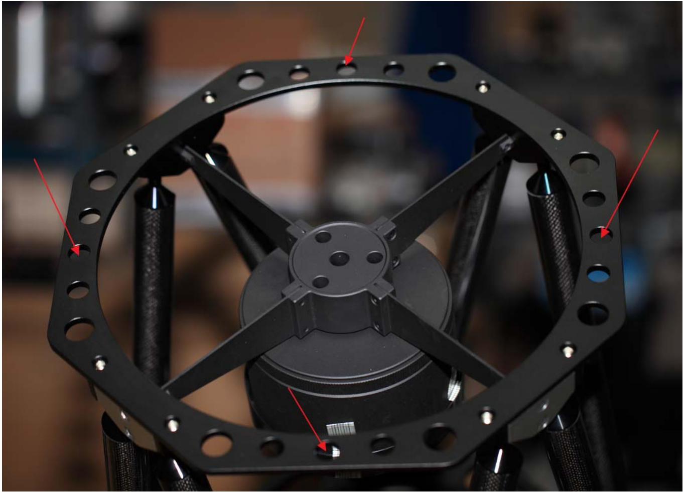
Fig. 5 Holes position for the DIMM mask
