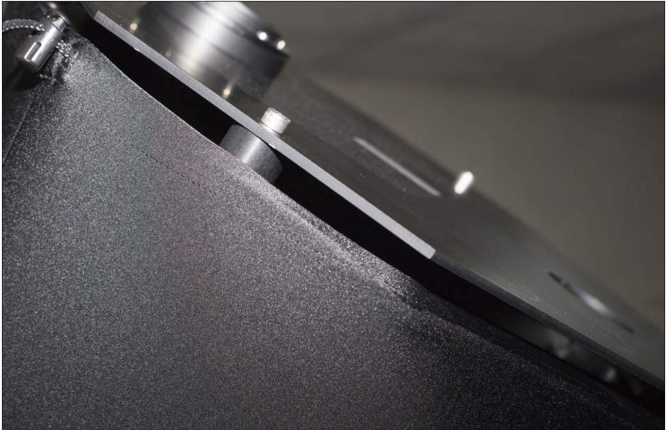
Fig. 11 Light shroud installation at the DIMM mask level
