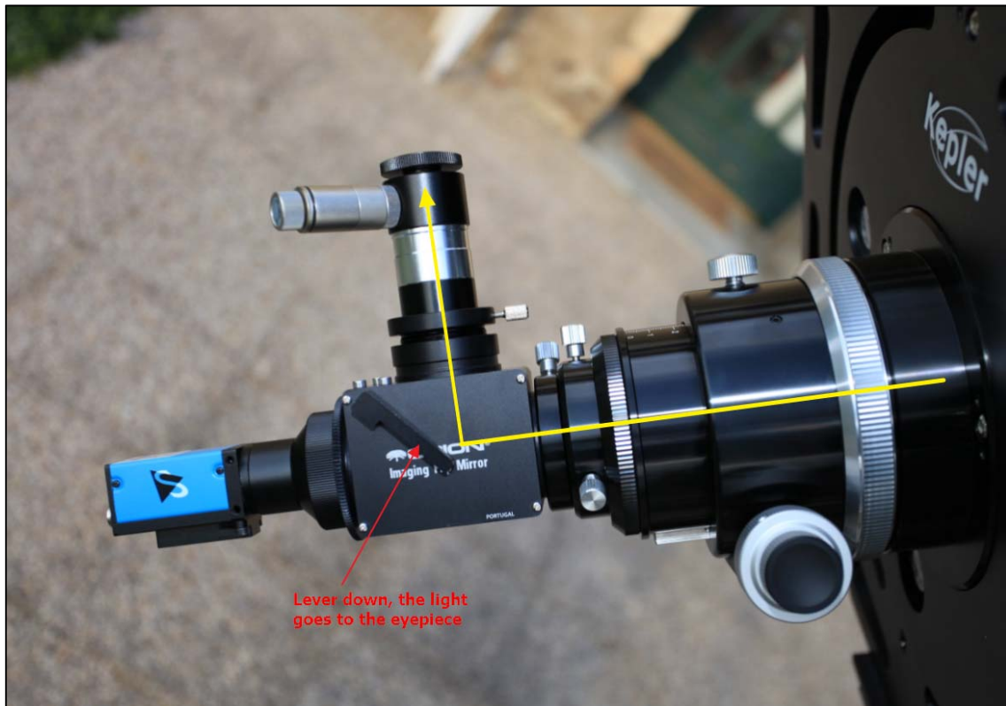
Fig. 13 DIMM camera, flip mirror and reticle eyepiece, light going to eyepiece
