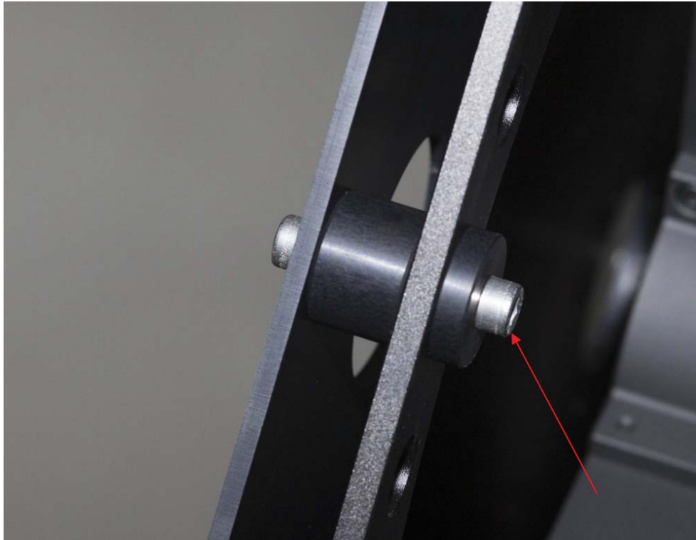
Fig. 6 DIMM mask installation on the telescope top ring
