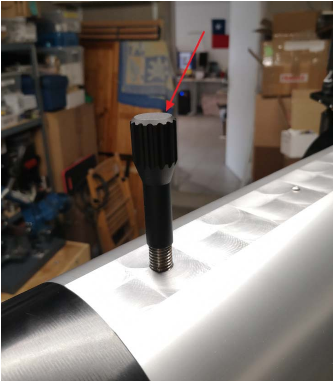
Figure 3 : Mount pin lock that prevent axis from rotating
