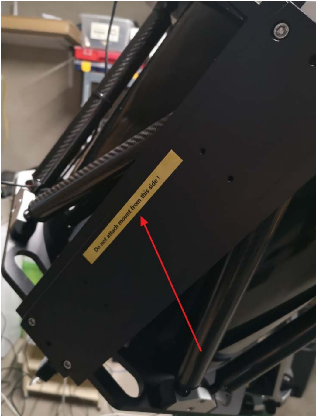
Figure 6 : The OTA must not be attached to the mount from this side.
