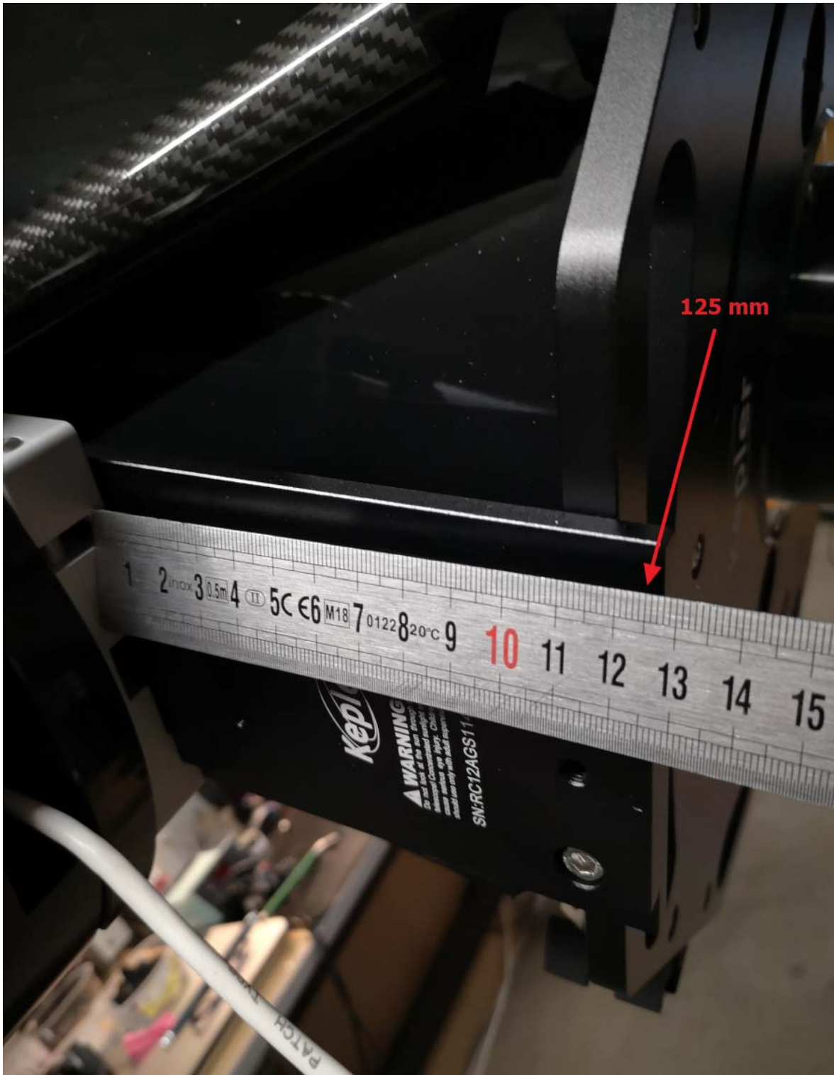
Figure 4 : The distance from the OTA backplate must be set to 125 mm
