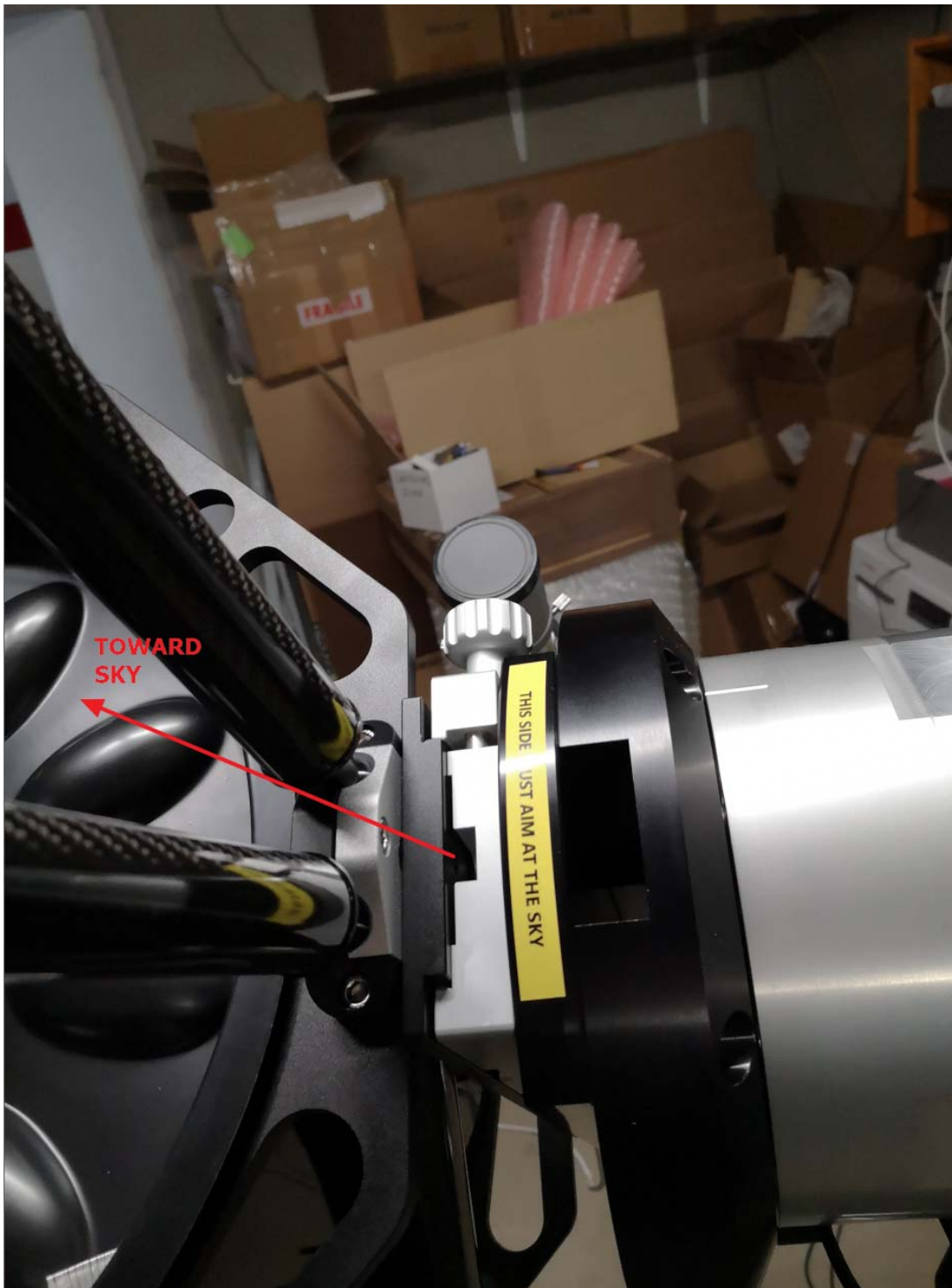
Figure 5 : The OTA light entrance must be located at the same side of the yellow sticker
