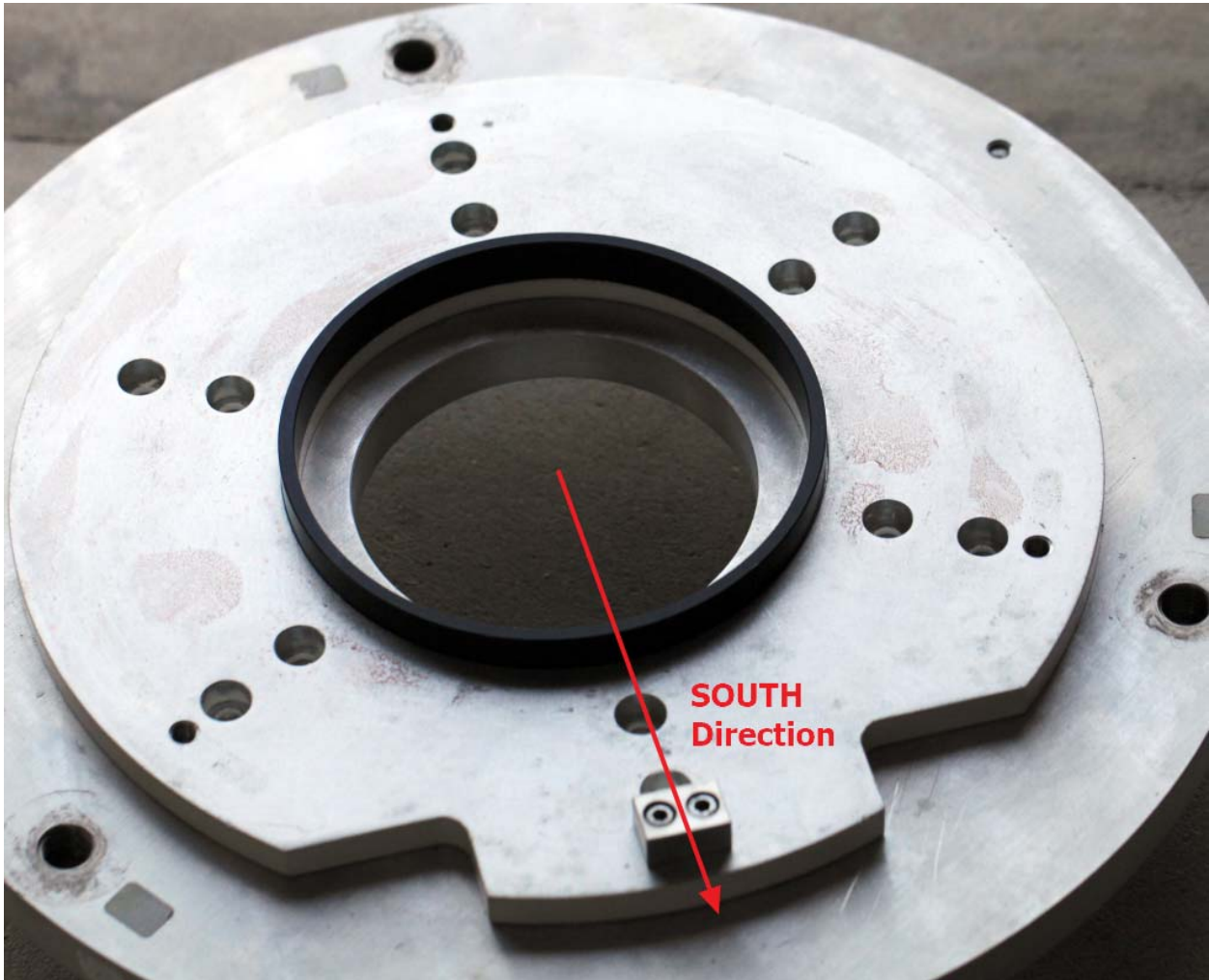
Figure 2 : Mount base plate must be oriented to the South this way.
