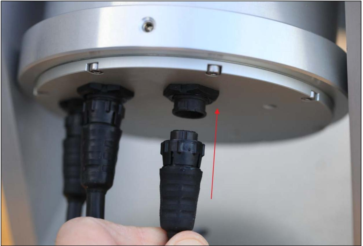
Fig. 8 Push the connector straight
