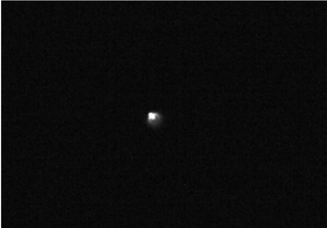
Fig. 67 Long exposure on Polaris (1/7s) showing some filter reflection effect (halo)
