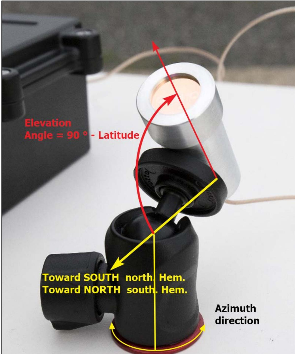
Fig. 10 Photodiode/sensor angle azimuth is set to north (or south) axis and elevation to  $90^\circ$  - latitude of the observing place.
