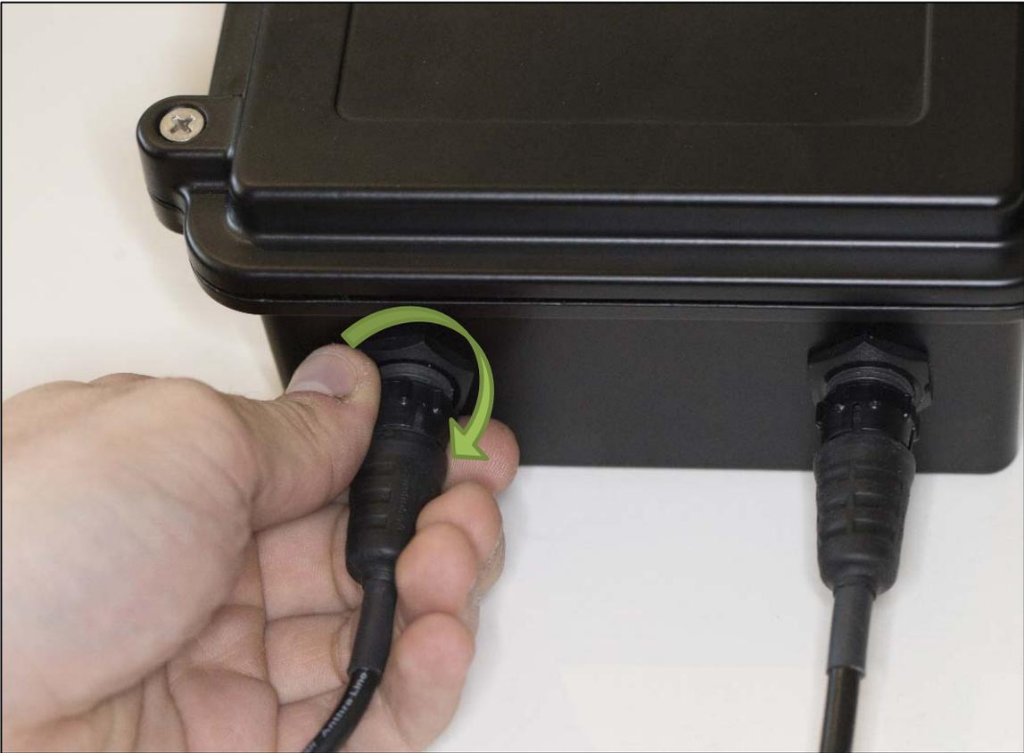
Fig. 7 Connector attachment step #2: rotate clockwise to have to lock the ring to prevent the cable from detaching
