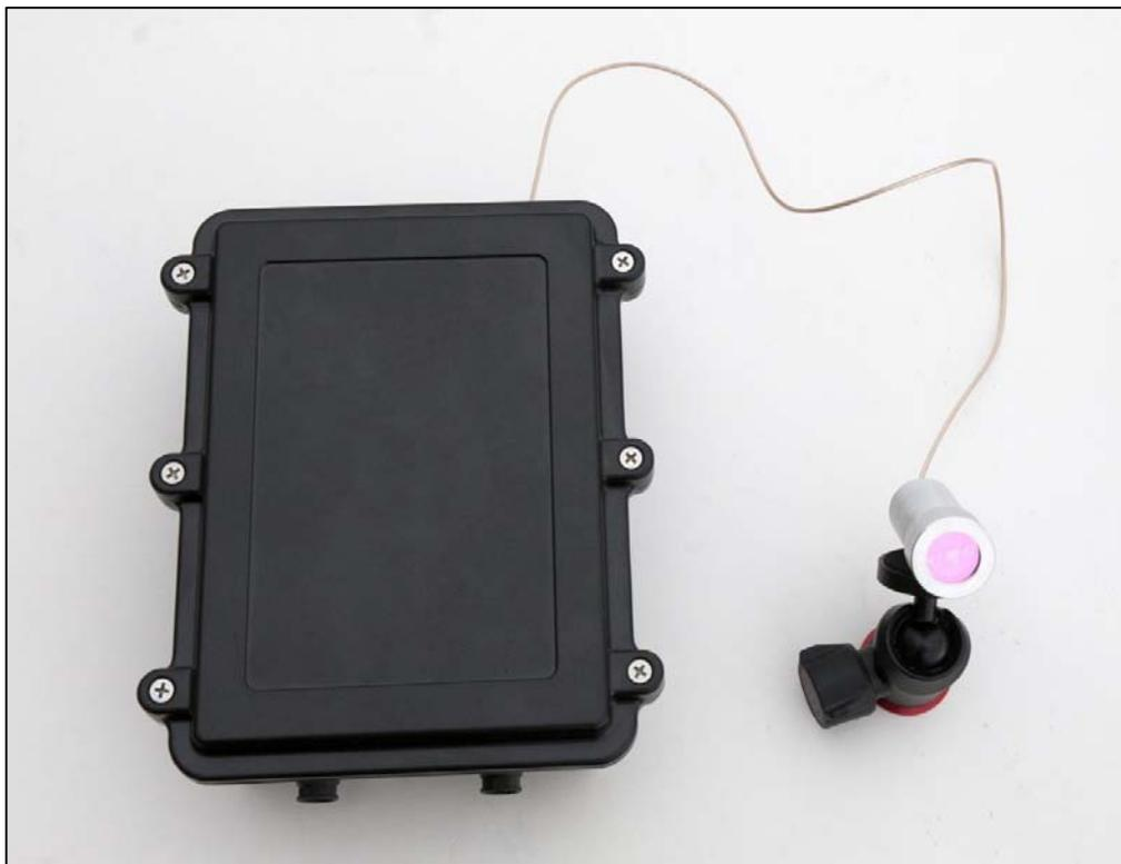
Fig. 1 Complete system without cables to computer and power supply, left main control box and right the sensor made of photodiode and green filter.
