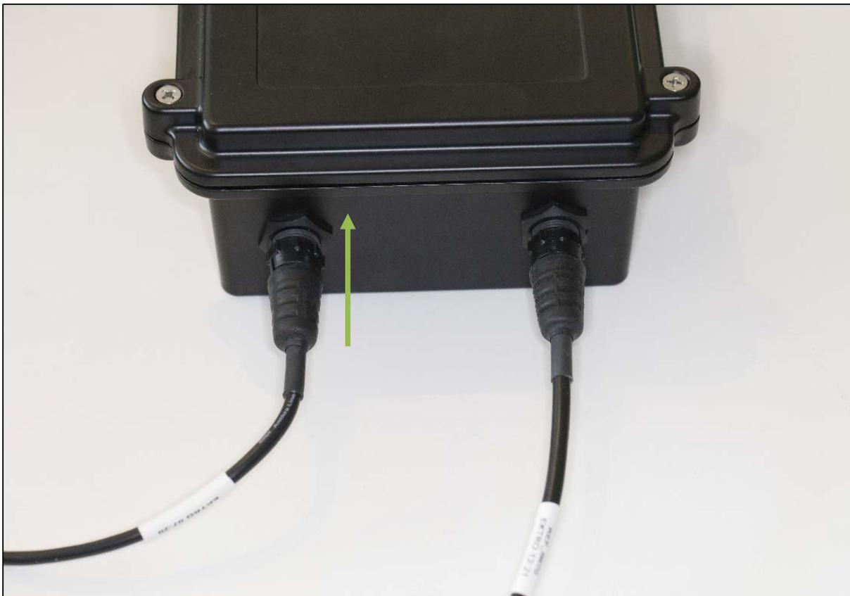
Fig. 6 Connector attachment step #1: go straight with proper key orientation
