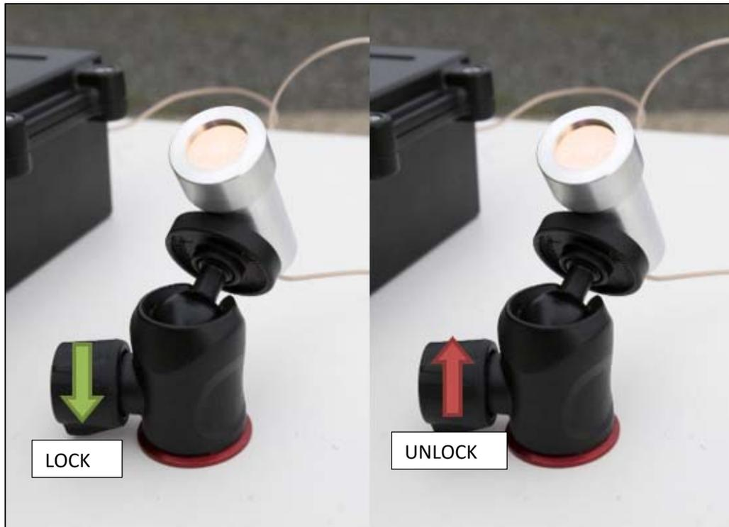
Fig. 11 Locking / Unlocking process of the elevation angle ball
